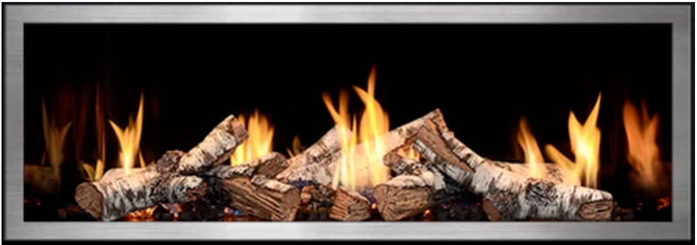
Figure 6-2 Burner Flame Heights: This image provides a visual reference for the burner flames burning at maximum height after the burners have been operating for 30 minutes or longer. This, however, is dependent on the gas type, air shutter opening setting and vent system configuration. Actual flame heights can be slightly higher or lower when compared to this reference image.
